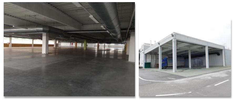
Total area: 8.700 m2 Office area (from the total area): 220 m2 Height of the structure: 4,60 m Load capacity of the structure: 400 kg/m2
